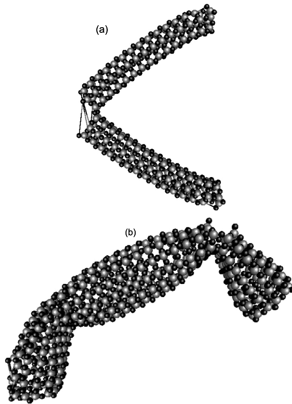
Figure 16. Fracture of (a) FB 6 M –30 L SWT, (b) FB 12 M –36 L SWT, under bending when subjected to a strain rate of 2.5 \times 10^{-4} \text{ ps}^{-1} at 10 K.
